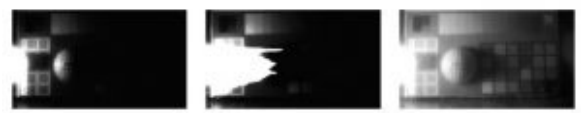
A scene with both 0000 bright and very dark components, imaged by .2 a standard IT-CCD (left), a standard EMCCD (center), and an Interline Transfer EMCCD device )(right
